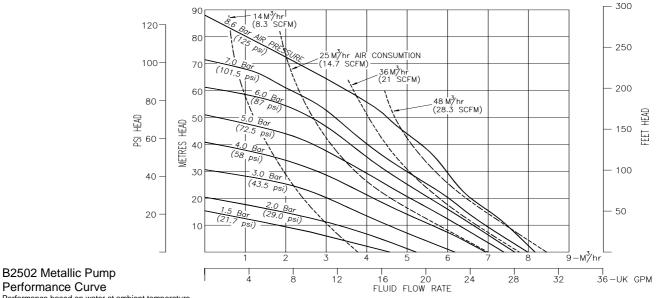
Performance based on water at ambient temperature
